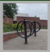
Description: A frame that is permanently anchored to the ground and is used to secure bikes when not in use. Bike racks should be located in visible areas and near major destinations such as employment centers,
