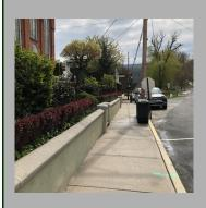
Description: Walkway parallel to the road that is intended for use by pedestrians, often with numerous access points to adjacent land uses. The walkway is typically physically separated from the roadway with a curb and/or verge. The verge may contain grass, vegetation, pavers,
