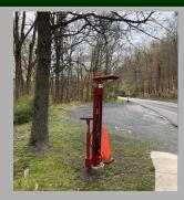
Description: A piece of equipment consisting of a simple bicycle stand and tools necessary to perform minor repairs and adjustments. The tools are typically securely attached to the stand, which can be use to hang the bike and allow the pedals and wheels to spin while making adjustments. Fix-It Stations should be located in visible areas,
