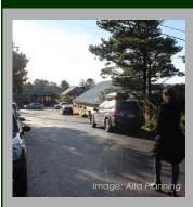
Description: A narrow roadway without pavement markings that is intended to support walking, biking, and driving in the low-speed travel way. These roads serve bi-directional traffic with no pavement markings,
