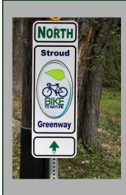
Description: Signs that can be stand alone or mounted on an existing pole that identify a facility and provide directional information, particularly at key decision points.
