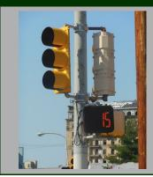
Description: Signal timings for pedestrians can include a leading pedestrian interval, which gives pedestrians a head start when entering an intersection. This enables pedestrians to establish their presence and
