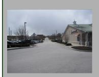
Description: Providing joint or cross access between adjacent properties allows circulation between the properties and reduces the number of driveways and conflict areas along a roadway. Joint and
