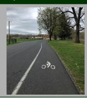
Description: A portion of the roadway that has been designated by striping, signage, and pavement markings for the preferential or exclusive public use by bicyclists. Bicycle lanes are located directly adjacent to motor vehicle travel lanes and operate in the same
