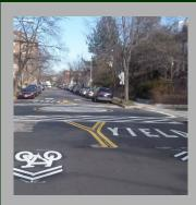
Description: Design treatments to offer priority for bicyclists operating within a roadway shared with motor vehicle traffic. Pavement markings, such as sharrows, and signage make users aware of the priority for bicycle travel and provide wayfinding. Can include traffic
