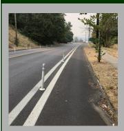
Description: A bicycle lane with a striped buffer area and vertical element that separates the vehicular travel lane and the shoulder used for the bicycle lane.
